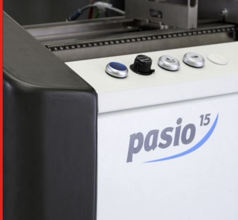
Mineral casting – robust and vibration-damping
